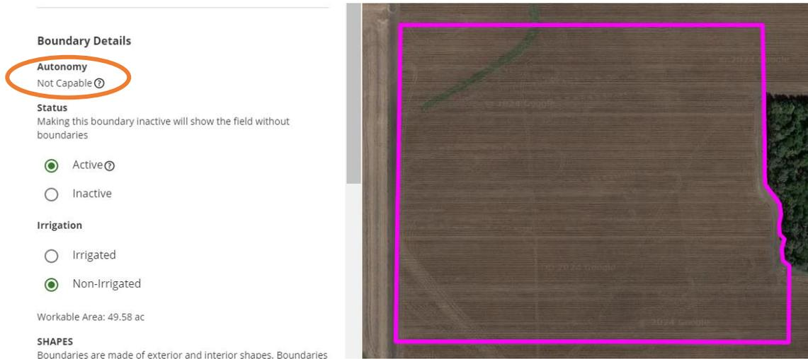
When creating a driven boundary, if any portion of the boundary is mapped in orange and any of the boundary recording checklist is not met, the boundary will be Not Autonomy Capable.
