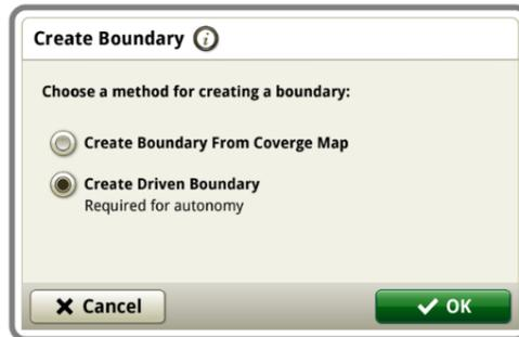
Many customers use a Gator equipped with the required technology to map boundaries. This allows for very precise movements around obstacles, curves, and corners to map the most accurate representation of the working area. Ensure that TCM Calibration has been completed prior to recording.
