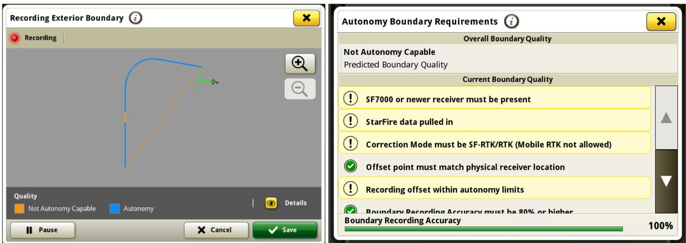
If creating a driven boundary using SF1, SF2, SF3, or mobile RTK signal, the entire boundary will be mapped in orange and will be Not Autonomy Capable.
