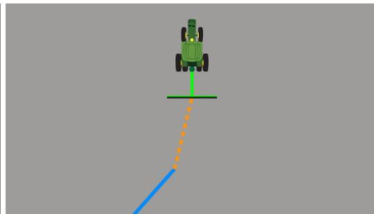
If you resume recording at this time, the orange portion of the boundary would be Not Autonomy Capable. If trying to achieve an Autonomy Boundary, return to a 5 meter distance from the pause point before resuming (indicated by blue dashes).
