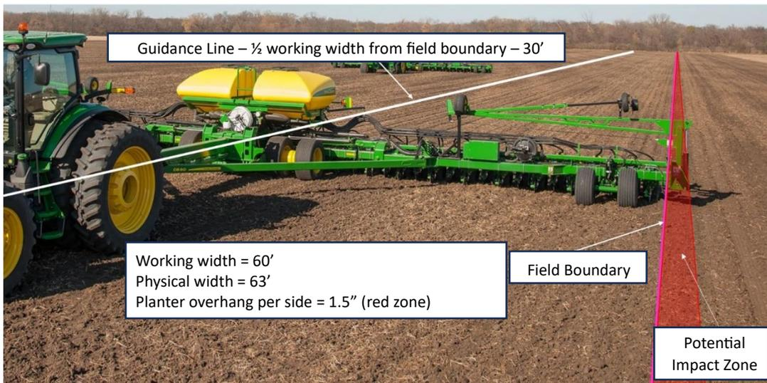
Some implements are wider than their working width. For instance, a planter may have a working width of 60', but a physical width of 63' due to the marker extensions. When recording a boundary, you must know and consider the extra width of the implement. Think about obstacles in/next to the edge of a field. You need to allow for that additional implement width to prevent machine damage.
