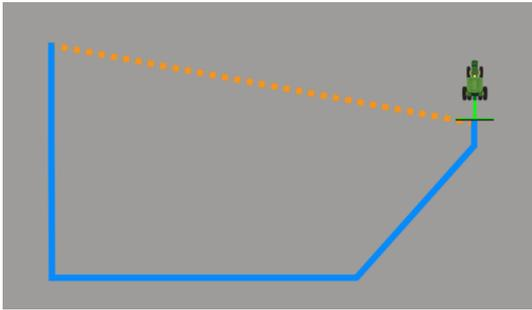
If saved at this time, the orange portion of the boundary would be Not Autonomy Capable meaning the entire boundary would be Not Autonomy Capable.
