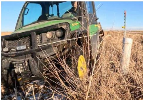
In the example on the left, a ‘safety rod’ or ‘buffer bar’ has been added to the front of the Gator. This gives the operator a visual reference as they drive and record a field boundary, of where any implement overhang, like the planter marker, will be located when traveling past an obstacle near the edge of the field.
