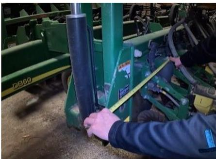
To accomplish this, measure how far the marker extension protrudes from the edge of the working width.
