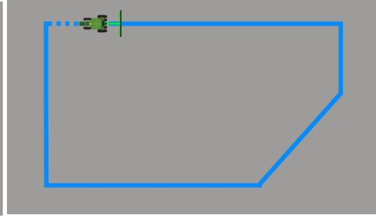
If the dashed line is blue, the distance between points is less than 5 meters and all prerequisites are met. If saved at this time, that portion of the boundary would be classified as Autonomy.
