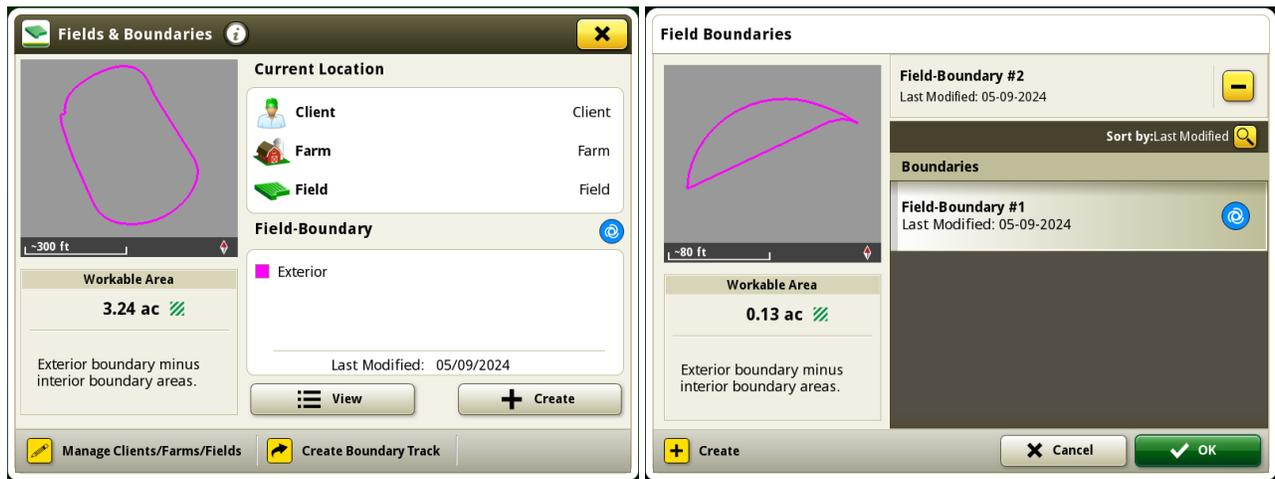
After saving a boundary, a blue Autonomy icon will be the indicator that the boundary achieves Autonomy quality requirements and is compatible for use with autonomous solutions.
