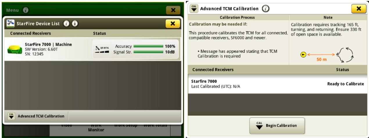
TCM calibration is specific to machine, so moving a receiver to a different machine will require the calibration to be done again. Additionally, anytime the receiver direction is changed or location on a machine is altered, the TCM calibration will need done again. If a DTC appears in the diagnostics center showing that the TCM has not been calibrated, you will see an unmet prerequisite appear in the details page showing that TCM must be calibrated.
