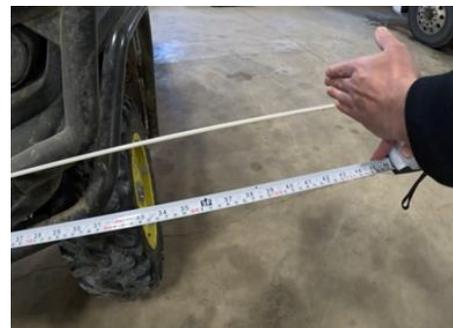
Similarly, this customer records the boundary at the left front tire, so the boundary is recorded wherever the outside of that tire drives.
